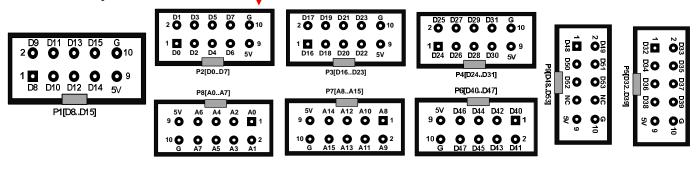
(JP1) = Jumper chooses the connection with Pin D19(Rx1), D18(Tx1) to run at Connector RS232-1 (support Board Mega1280,2560) or at Connector Port P3, please set Jumper as shown below;
