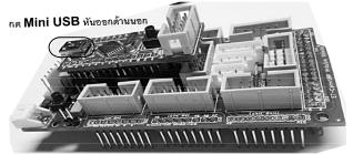
**Con-Arduino UNO** = This is position of Connector MALE to connect to Board MCU Arduino UNO. First of all, please look at Pin Mark's position on both sides of Board Shield that must correspond with Pin A5 and D0 of Board MCU Arduino; next, carefully place the board and slightly push down Pins as shown in the picture.
