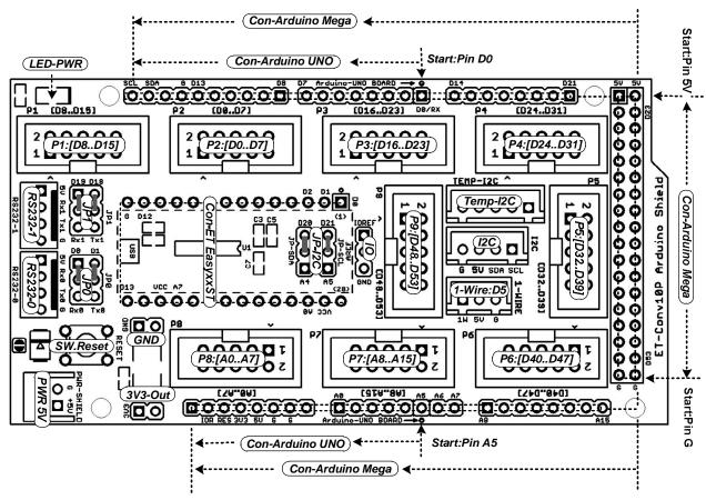
(LED-PWR) = LED shows status of connecting Power 5V to Connector Power of Board Shield or connecting to Power Supply of Board MCU.
